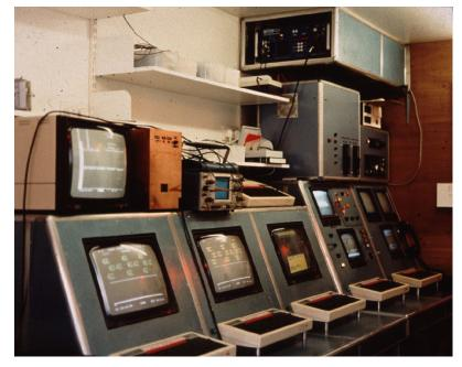
**Figure 4.** The Durham Mark III telescope control room. While the main DAQ was performed by a Motorola 68000 computer situated under the console, the system's interfaces were all BBC microcomputers. These were remarkable- and remarkably cheap-computers for their time. The copper box on top of the console contains the rubidium oscillator used for timing.
