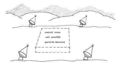
**Figure 1.** The 'third generation' gamma-ray telescope array proposed by Turver and Weekes [5]. The suggested energy range was 10 Gev to 10 TeV; each reflector would be 10–15 m in diameter and be separated by 50–100 m.
