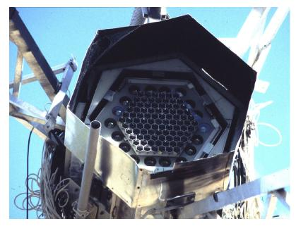
Figure 6. The Durham Mark 6 telescope's central camera.
