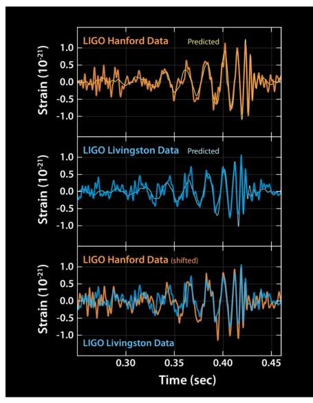
The observed GW signal from the two LIGO interferometers is shown in Figure 3.
