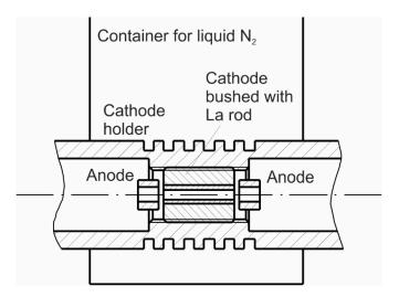
**Figure 1.** Sketch of the hollow cathode lamp. The ceramic anode holders and the connecting pins are not shown. The cathode holder is grounded. Length of the cathode is 20 mm.
