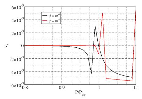
**Figure 8.** Comparison of the photon component  $v_n$  of the least stable eigenvector (matching the least stable eigenvalue in Figure 4) for a micro- ( $\beta = 10^{-4}$ ) and a macroscopic laser ( $\beta = 10^{-6}$ ). As in Figure 7, each curve stops at the point where the eigenvector becomes complex, simultaneously with the appearance of an imaginary component in the corresponding eigenvalue.
