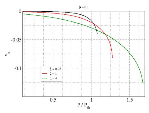
**Figure 11.** Normalized photon component  $v_n$  of the least stable eigenvector (matching the least stable eigenvalue in Figure 10) for different kinds of asymmetry in the emission rates. Each curve stops at the point where the eigenvector becomes complex, simultaneously with the appearance of an imaginary component in the corresponding eigenvalue.  $\beta = 10^{-1}$ .
