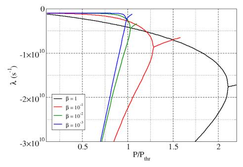
**Figure 4.** Real part of the eigenvalues derived from the stability analysis of the rate equations model, Equations (12) and (13). The different curves belong to different values of the fraction of spontaneous emission coupled into the lasing mode (cf. figure legend).
