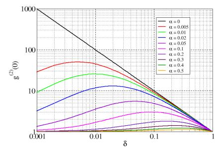
**Figure 3.** Zero-delay second-order autocorrelation, Equation (4), in double logarithmic scale, as a function of the duty cycle  $\delta$ , and for different values of the baseline's amplitude  $\alpha$  (fraction of the peak amplitude *A*).
