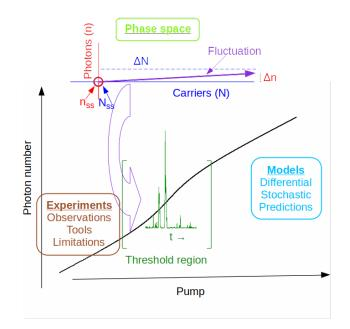
**Figure 1.** Graphical representation of the topics addressed in the manuscript.  $N_{ss}$  and  $n_{ss}$  refer to the steady-state operation values of the population inversion and photon number, respectively, around which a fluctuations operates, for a given set of parameters.
