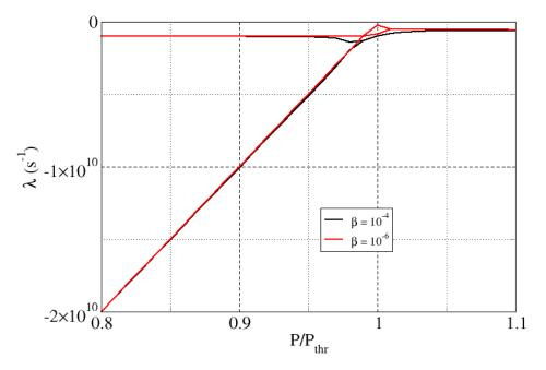
**Figure 6.** Real part of the eigenvalues derived from the stability analysis of the rate equations model, Equations (12) and (13) for a borderline microlaser ( $\beta = 10^{-4}$ ) and for a macroscopic laser  $\beta = 10^{-6}$ )—cf. figure legend.
