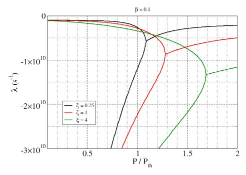
**Figure 10.** Real part of the eigenvalues derived from the stability analysis of the modified rate equations model, Equations (16) and (17). The different curves belong to different kinds of asymmetry (cf. figure legend).  $\beta = 10^{-1}$ . The chosen values of  $\xi$ , here and in the following figure, are those of [104].
