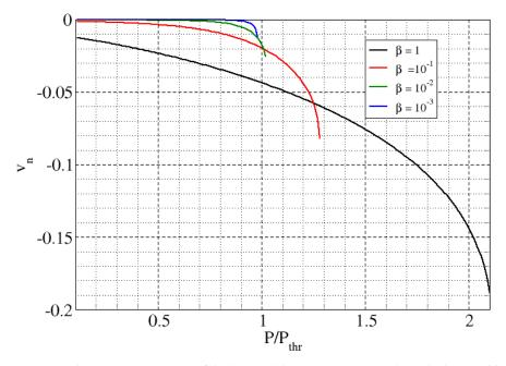
**Figure 7.** Photon component  $v_n$  of the least stable eigenvector (matching the least stable eigenvalue in Figure 4) for differently-sized lasers. Each curve stops at the point where the eigenvector becomes complex, simultaneously with the appearance of an imaginary component in the corresponding eigenvalue.
