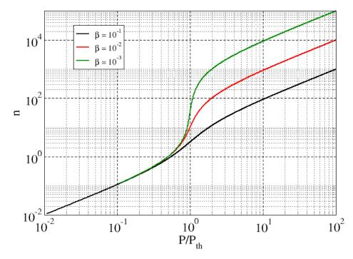
**Figure 5.** Laser characteristic response in double-logarithmic scale as a function of normalized pump, for different values of  $\beta$  (cf. legend).
