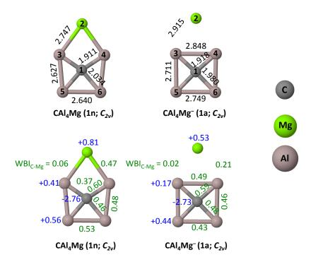
**Figure 1.** Global minimum structures of CAl<sub>4</sub>Mg (**1n**) and CAl<sub>4</sub>Mg<sup>-</sup> (**1a**). Bond lengths are given in Å in the top row. The atom numbering scheme used herein is also shown. Natural atomic charges (in |e|; blue color) and Wiberg bond indices (green color) calculated at the (U) $\omega$ B97XD/6-311++G(2d,2p) level are given in the bottom row.
