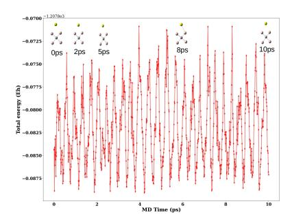
**Figure 11.** Energy evolution of CAl<sub>4</sub>Mg<sup>-</sup> (**1a**) at 298 K in 10 ps ab initio MD simulations calculated at the U $\omega$ B97XD/6-311++G(2d,2p) level.
