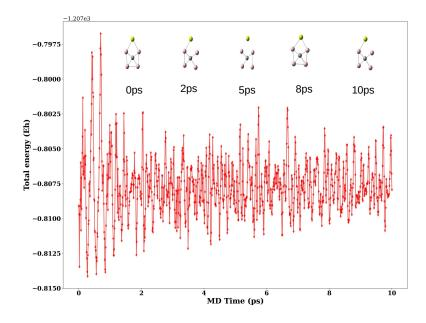
**Figure 10.** Energy evolution of CAl<sub>4</sub>Mg (1n) at 298 K in 10 ps ab initio MD simulations calculated at the  $\omega$ B97XD/6-311++G(2d,2p) level.
