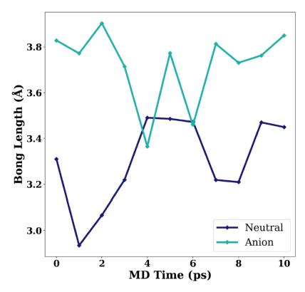
**Figure 9.** Bond length (C-Mg) evolution of CAl<sub>4</sub>Mg (**1n**) and CAl<sub>4</sub>Mg<sup>-</sup> (**1a**) at 298 K in 10 ps ab initio MD simulations calculated at the (U) $\omega$ B97XD/6-311++G(2d,2p) level.
