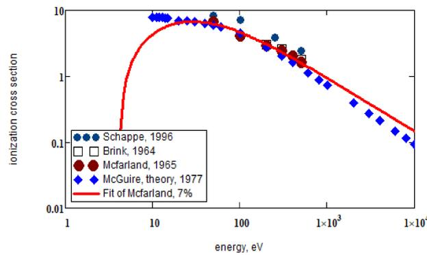
Figure 5. Electron impact ionization cross sections of rubidium in Å<sup>2</sup>.
