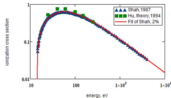
**Figure 1.** Electron impact ionization cross sections of hydrogen in  $\text{\AA}^2$ .
