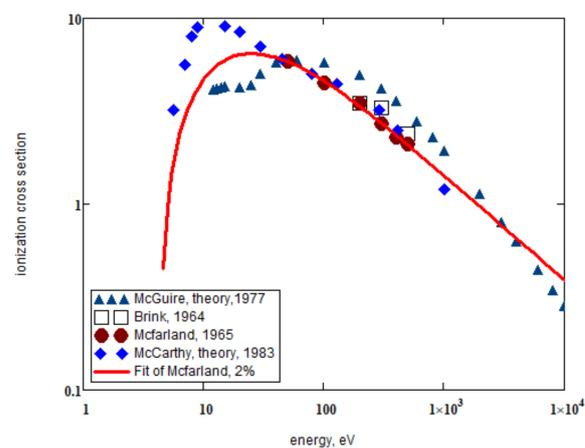
Figure 4. Electron impact ionization of potassium in  $\text{\AA}^2$ .
