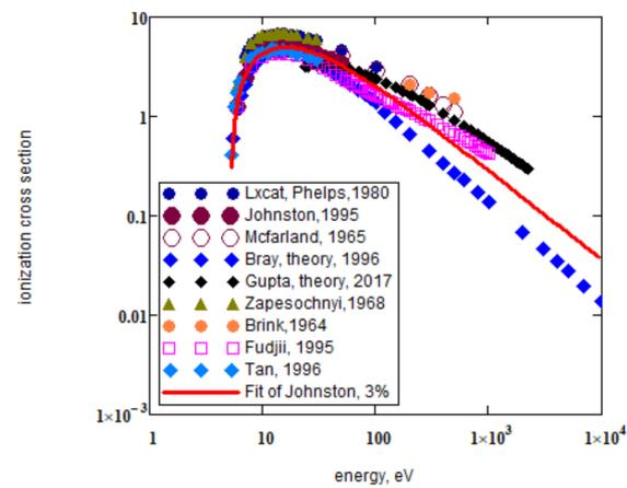
Figure 3. Electron impact ionization cross sections of sodium in  $\text{\AA}^2$ .
