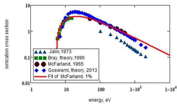
Figure 2. Electron impact ionization cross sections of lithium in  $\text{\AA}^2$ .
