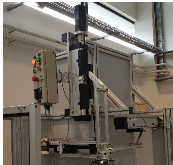
Figure 2. The prototype of the Orthoglide (LS2N).
