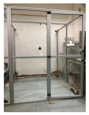
Figure 5. Prototype cable suspended parallel robot (CSPR) used during the tests.
