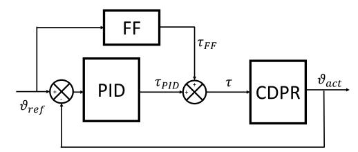
Figure 2. PID and feed-forward control scheme of the robot.
