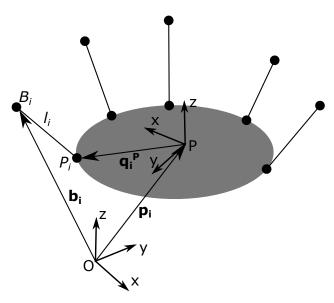
Figure 1. Example of a generic suspended cable-driven parallel robot.
