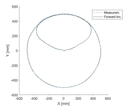
**Figure 7.** Spatial trajectory of the end-effector: comparison between the reference motion (actuator position) and the measurements from the motion tracking system.
