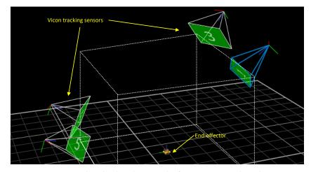
**Figure 6.** Vicon Tracker display showing the four cameras and markers position with respect to the robot workcell. FoV: field of view.
