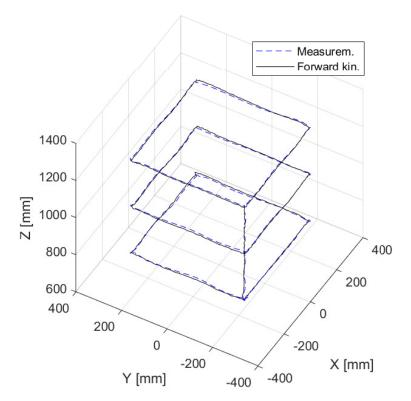
**Figure 9.** Comparison between the reference motion (actuator position) and the measurements from the motion tracking system using a more complex trajectory.
