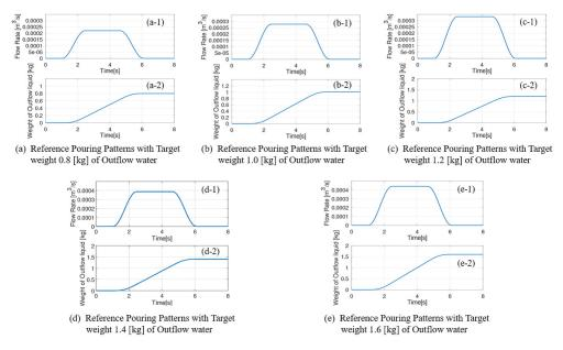
Figure 14. Pouring Patterns as Reference Input in Experiments.
