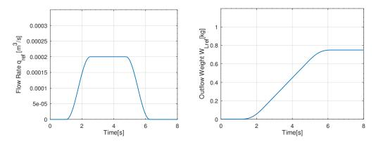
Figure 10. Desired pouring patterns.
