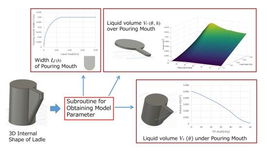
Figure 11. Derivation system of model parameters from ladle shape.
