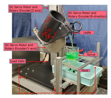
Figure 2. Tilting-ladle-type automatic pouring machine in laboratory.
