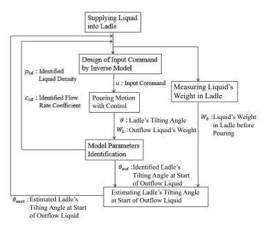
Figure 13. Flowchart of updating controller's parameters.
