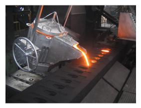
Figure 1. Tilting-ladle-type automatic pouring machine.
