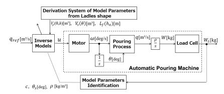
Figure 8. Block diagram of proposed pouring flow rate control system.
