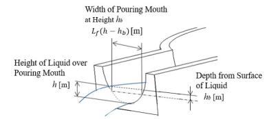
Figure 6. Parameters on pouring mouth.
