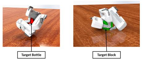
**Figure 4.** Various grasp pose configurations for bottle and block targets. Bottle targets are symmetric in x and y compared to blocks which are symmetric in x, y, and z.
