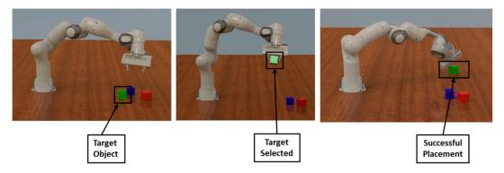
Figure 1. Pick-and-place of color-coded square blocks with the Franka Emika Panda robot.
