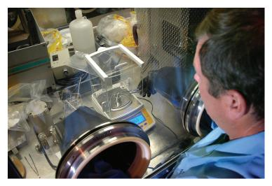
**Figure 1.** A nuclear glovebox where the access to the interior is through the glove ports. The operator is wearing the specially designed gloves to protect himself from contamination. Source: Wikimedia Commons.
