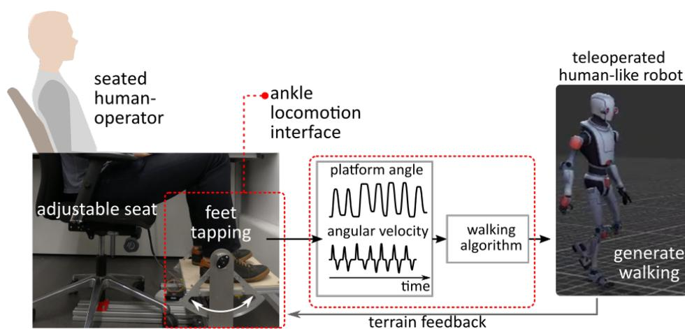
**Figure 11.** Teleoperation system based on seated ankle interface to control locomotion of remote mobile robotic systems. A human operator uses feet tapping movements to control the walking of a humanoid robot, i.e., its gait. Terrain feedback from a remote environment is rendered to a human operator.
