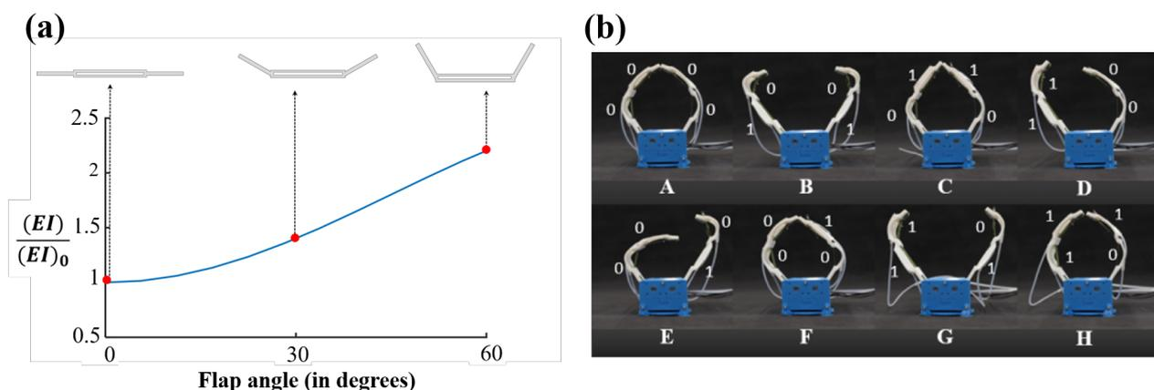
**Figure 3.** (a) Variation of flexural stiffness as a function of the flap angle. (b) Actuation of different pouches leads to different gripper configurations upon actuation by tendons (Reprinted with permission from ref. [19]. Copyright 2020 IEEE).
