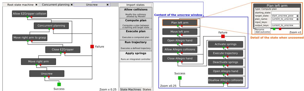
**Figure 6.** The appearance of the task editor when designing a bimanual operation. The user can navigate both between and within hierarchies, via the sub-windows that are created when new containers are added. Different levels of zoom will show or hide the configuration data of each state, to ensure an appropriate visualisation (Reprinted with permission from ref. [27]. Copyright 2020 IEEE).
