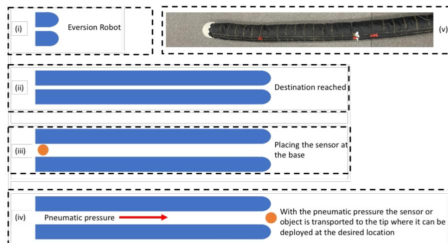
**Figure 8.** The two ways an eversion robot can deliver sensors in an unknown environment. (i–iv) Passing the sensor load through the central chamber of the eversion robot. (v) Cap mounted on the eversion robot's tip to which sensor load can be attached for transportation as growth occurs.
