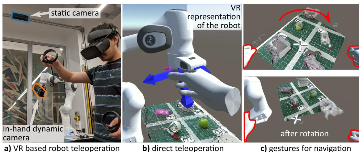
**Figure 9.** Overview of the proposed virtual reality-based robot teleoperation. (a) A human operator uses VR to command a robot. (b) A human operator's view of the VR representation of the robot and its environment used for direct teleoperation. (c) Hand gestures used for rotating and scaling the VR scene. (Reprinted with permission from ref. [73]. Copyright 2020 IEEE).
