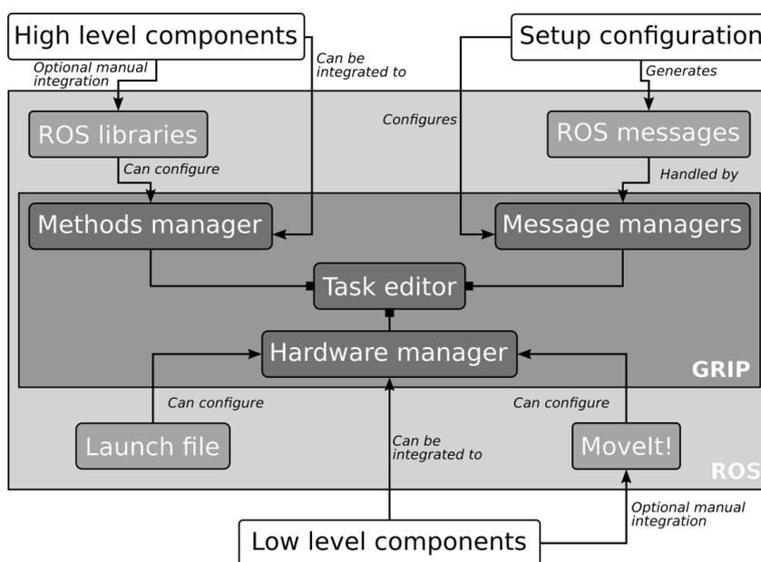
**Figure 4.** Overview of the GRIP framework. The architecture allows users to operate robots with integrated components (hardware and/or software) for grasping and manipulation tasks. The task editor provides an intuitive interface for designing and tuning the robot’s behaviour. Arrows indicate the different (mutually compatible) ways to interface external components (Reprinted with permission from ref. [27]. Copyright 2020 IEEE).
