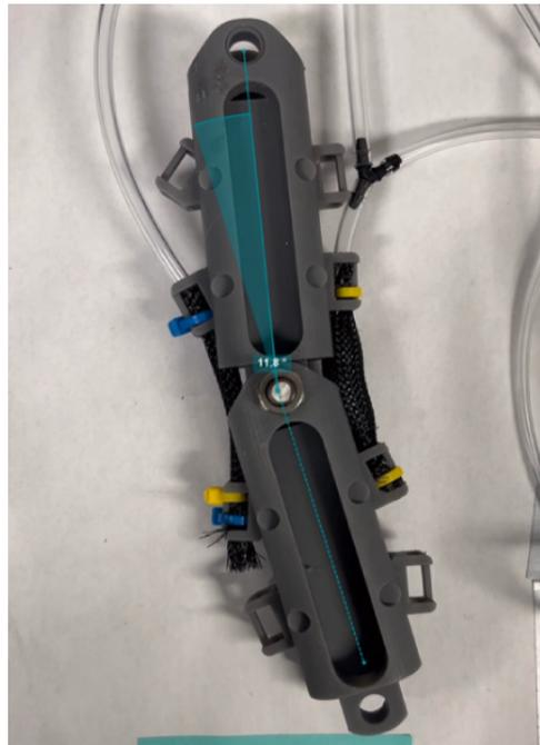
**Figure 12.** A single module of muscle-driven mechanism for the control test.
