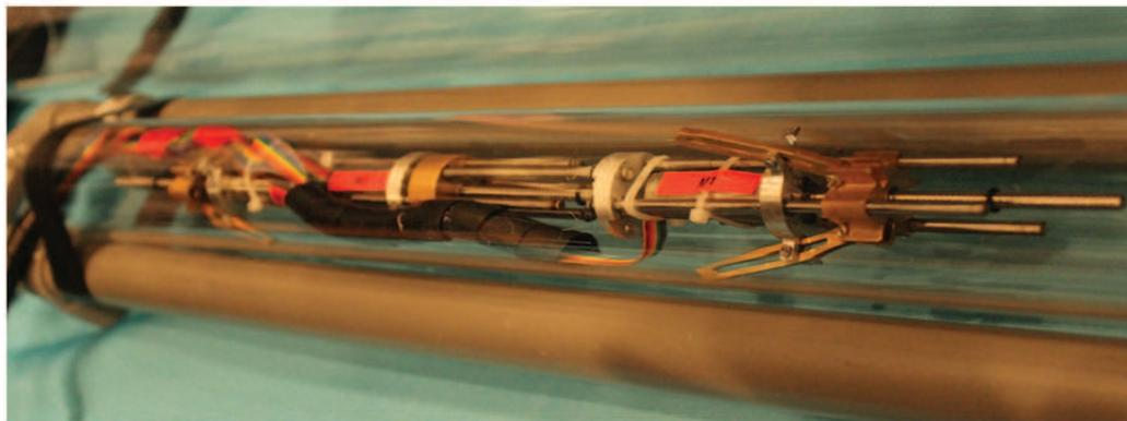
**(A) Working of the robot inside the PVC test pipeline**
