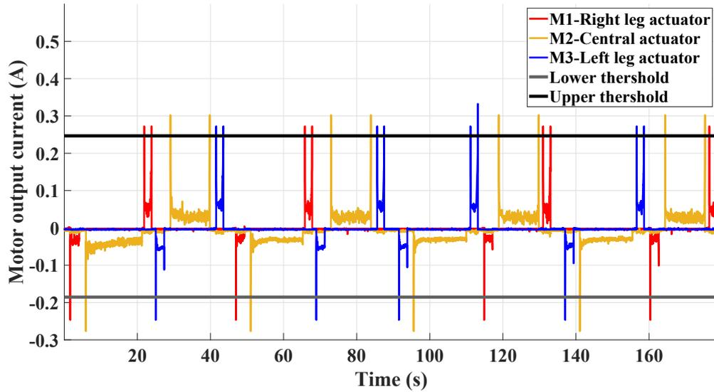
Figure 10. Output current of EC-motors from experiments.
