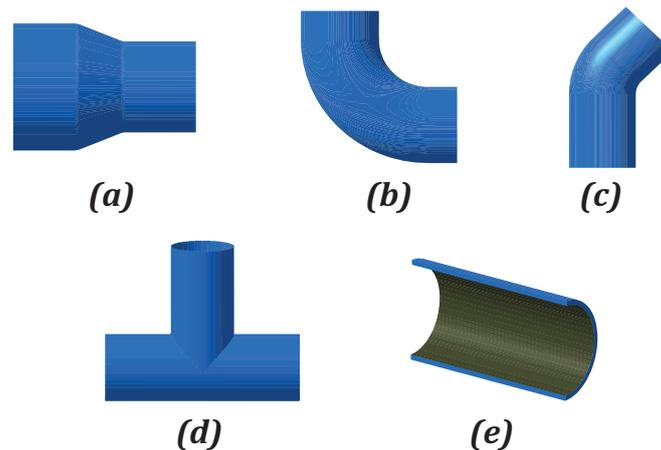
**Figure 6.** Possible profiles encountered by an inspection robot inside an industrial pipeline: (a) varying diameter; (b) curvature; (c) inclination; (d) branching; and (e) uneven surface walls [21].
