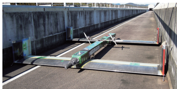
Figure 17. The experimental WIG effect vehicle ARTE02 [16].
