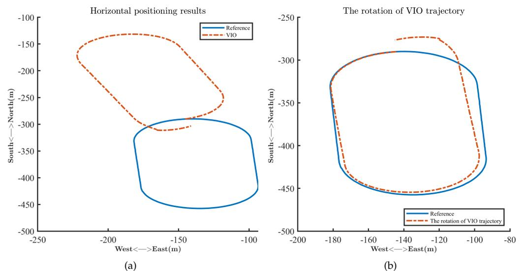
**Figure 13.** The performance of the standalone visual–inertial odometry (VIO). (a) The trajectory given by the standalone VIO. (b) The rotation of VIO's trajectory.
