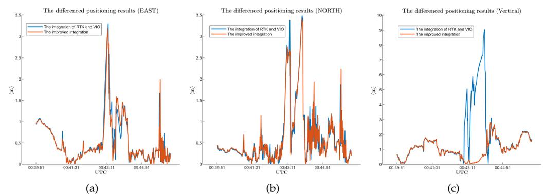
Figure 19. The differences between the reference and the integration results of different strategies. (a) The differences between the reference and the integration results in east. (b) The differences between the reference and the integration results in north. (c) The differences between the reference and the integration results in vertical.
