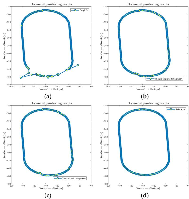
**Figure 20.** The performances in continuity of different algorithms. (a) The valid positioning results of RTK. (b) The valid positioning results of the pre-improved integration. (c) The valid positioning results of the improved integration. (d) The reference.
