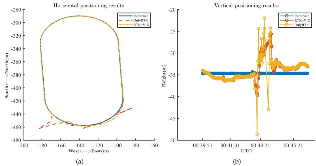
**Figure 14.** The performance of the integration of real-time kinematic (RTK) technique and VIO. (a) Horizontal positioning results. (b) Vertical positioning results.
