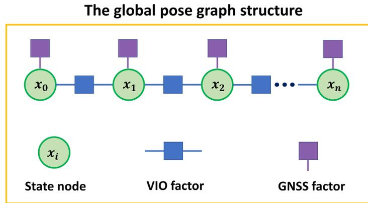
**Figure 4.** The global pose structure of VINS-fusion.
