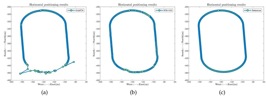
**Figure 15.** The performance comparison of RTK, RTK/VIO, and the reference. (a) Valid positioning results of RTK. (b) Valid positioning results of RTK/VIO. (c) The reference.
