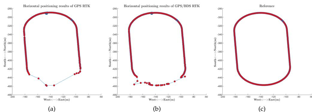
**Figure 12.** The performance comparison of GPS RTK, GPS/BDS RTK, and the reference. (a) Horizontal positioning results of GPS RTK. (b) Horizontal positioning results of GPS/BDS RTK. (c) The reference.
