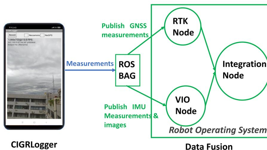
Figure 6. The CIGRLogger and the flow chart of the software design.
