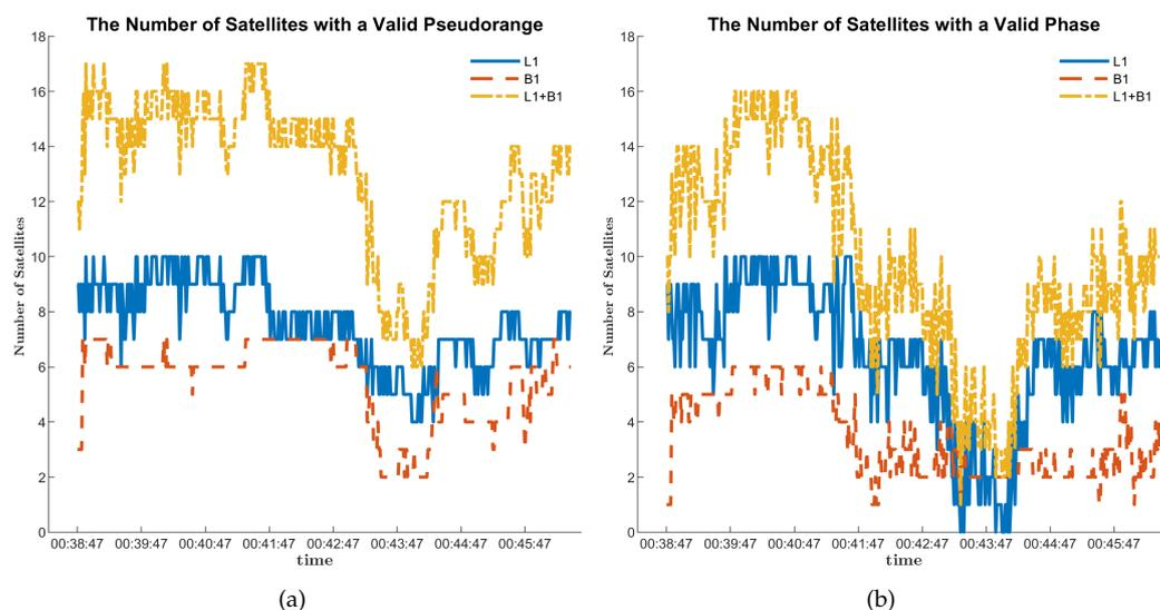
**Figure 11.** The number of the visible satellites with a valid pseudo-range and the number of the visible satellites with a valid carrier phase at different moments. (a) The number of the visible satellites with a valid pseudo-range at different moments. (b) The number of the visible satellites with a valid carrier phase at different moments.
