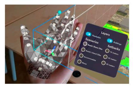
**Figure 7.** Screenshot of a single user application in use, with the content menu activated by bringing up the palm. You can see the hand mesh visualization, providing visual feedback to the user. Note: the significant displacement/difference between virtual and real hand only appears on captured videos/screenshots.
