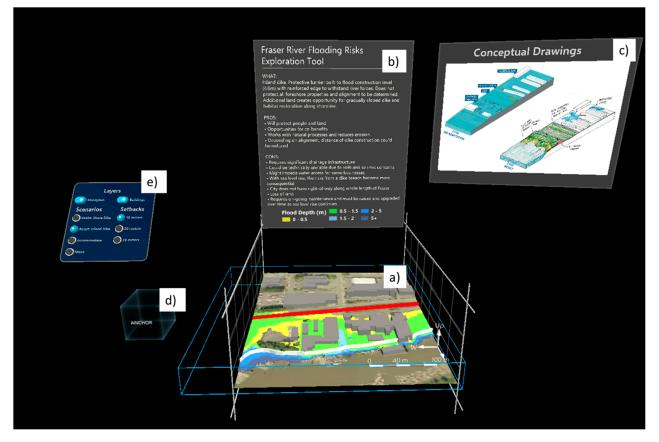
**Figure 3.** This screenshot captures the developed UI (user interface) of the visualization in a shared application, with an inland dike adaptation scenario selected: (**a**) 3D content, with 2 clipping planes, scale bar and directional arrows; (**b**) text panel providing vis. and scenario description; (**c**) conceptual drawings related to a scenario; (**d**) Anchor object used to synchronize position; (**e**) content menu.
