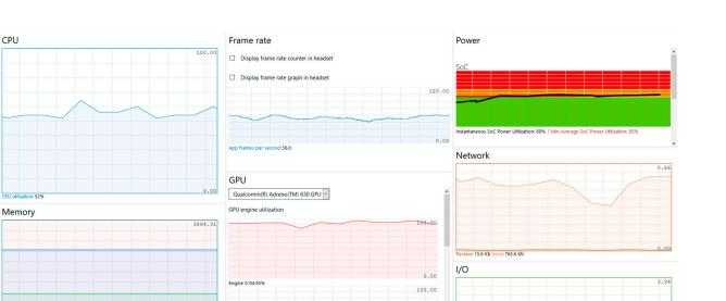
Figure 5. Screenshot of a live hardware usage of shared MR (mixed reality) visualization. As you can see, the usage of CPU (central processing unit) is at 50–60%, and GPU load fluctuates at almost 100%, with framerates fluctuating between 50–60 fps, which is sufficient for smooth application performance.
