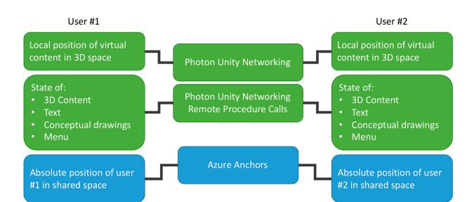
**Figure 4.** This chart illustrates how the various components of the shared experience are synchronized across two users, with Photon Unity Networking and Remote Procedural calls connecting the content state across two users, and Azure Anchors providing the common coordinate system for to users.
