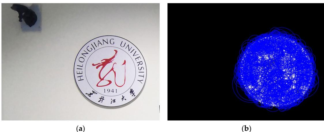
**Figure 10.** Foreground feature extraction based on ARAC. The feature points extracted from the foreground area are represented by blue circles: (a) origin image; (b) ARAC foreground feature.
