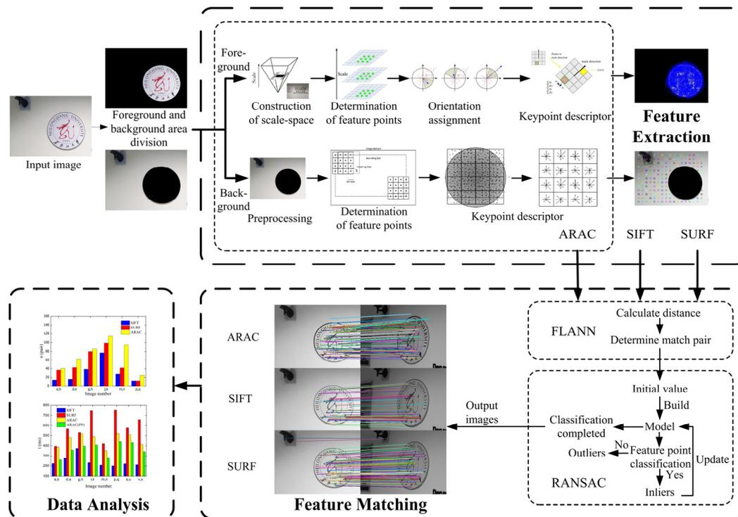
**Figure 1.** Roadmap of the research. In the data analysis, blue, red, yellow, and green represent SIFT, SURF, ARAC, and ARAC under parallel processing, respectively.
