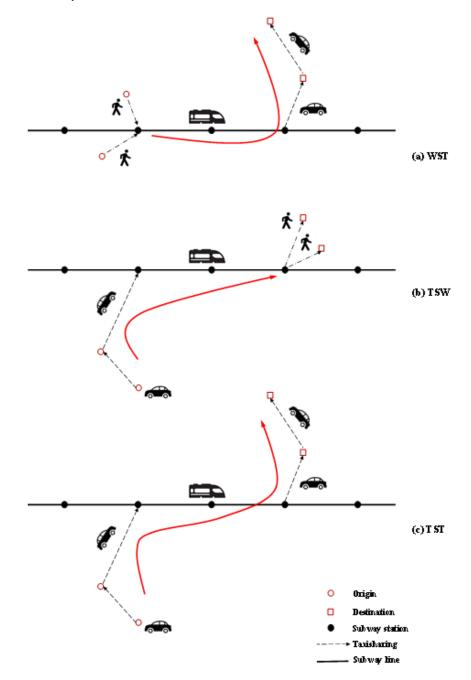
**Figure 1.** Illustration of three subtypes of taxi-sharing and subway multimodal transportation including (**a**) WST (**b**) TSW and (**c**) TST.
