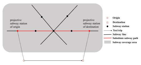
Figure 2. Illustration of alternative subway path.
