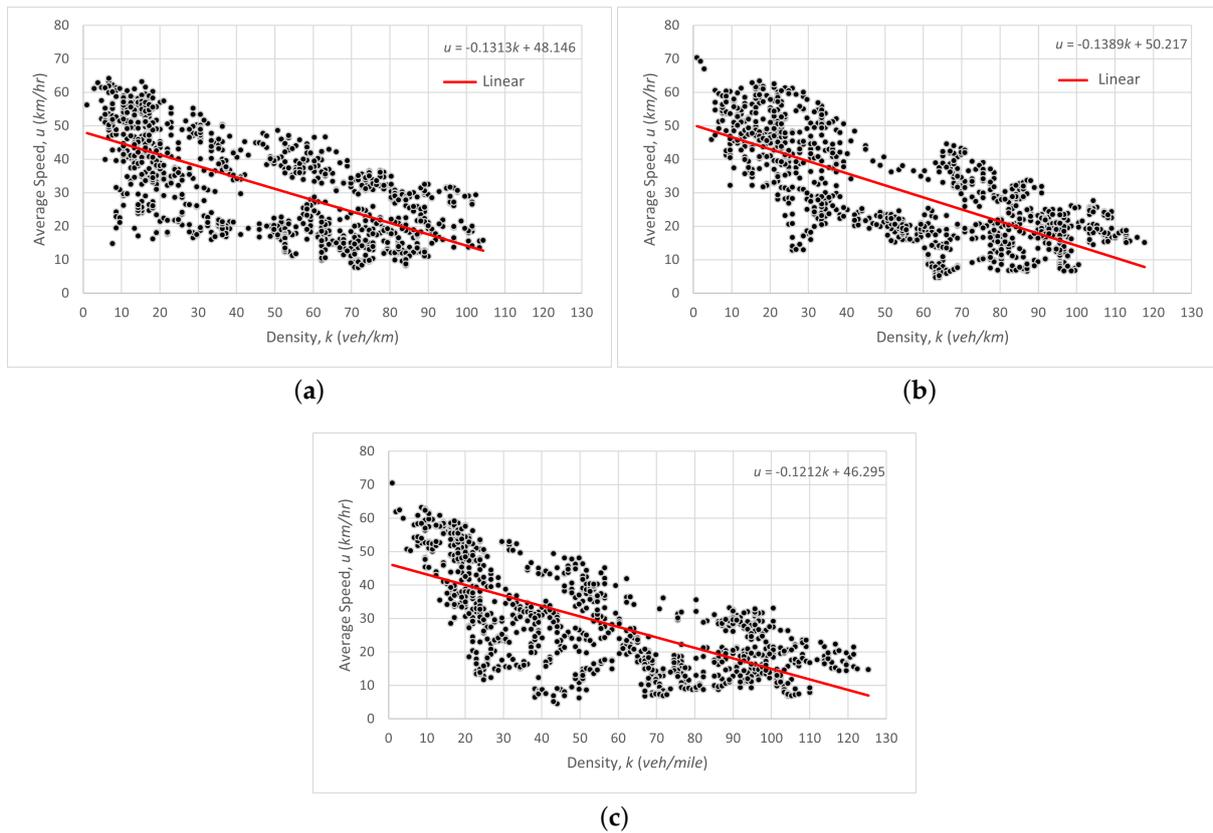
**Figure 18.** The average speed of the vehicle against density during peak hour for 20 s, 30 s and 40 s duration of green light. (a) 20 s duration of green light. (b) 30 s duration of green light. (c) 40 s duration of green light.
