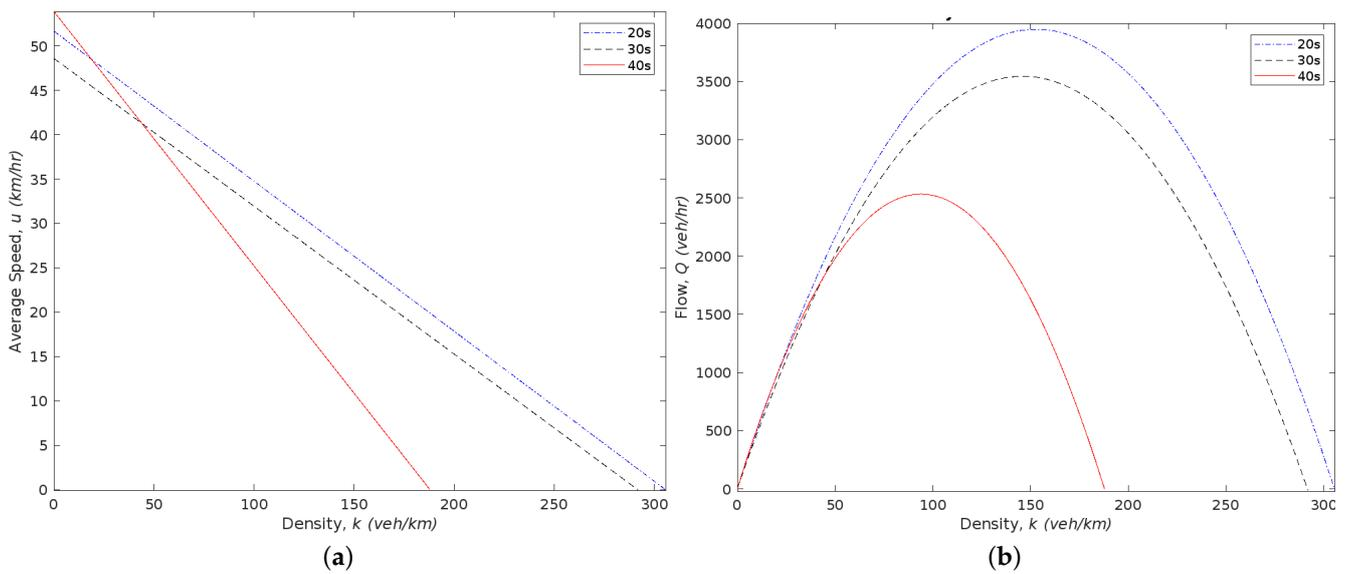
**Figure 15.** Speed-density and flow-density relation during the off-peak hour for different traffic light phasing. (a) Speed-density relation. (b) Flow-density relation.
