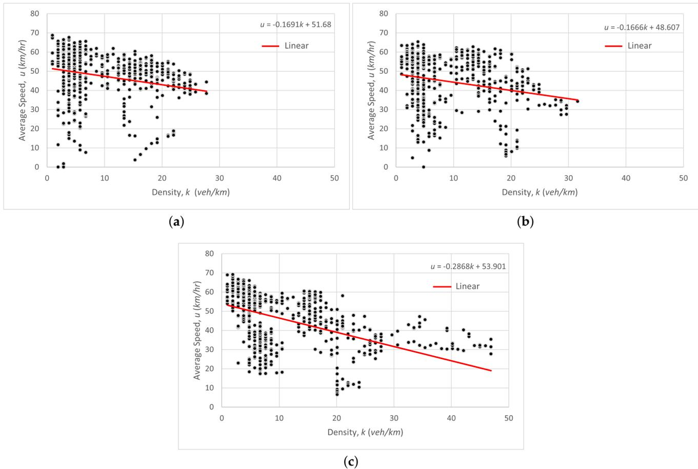
**Figure 14.** Results on the collected data of density and average speed during the off-peak hour for 20 s, 30 s and 40 s duration of green light. (a) 20 s duration of green light. (b) 30 s duration of green light. (c) 40 s duration of green light.
