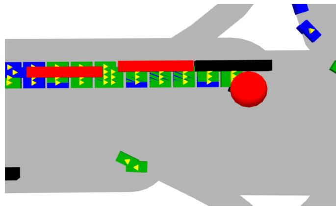
**Figure 7.** The 3D display of moving vehicle agents represented in cuboid shape on the road network in the GAMA simulation platform (blue: people, green: wanderer, red: bus, black: lorry). The yellow triangle indicates the direction of movement, and the red sphere is the stop signal (the traffic lights).
