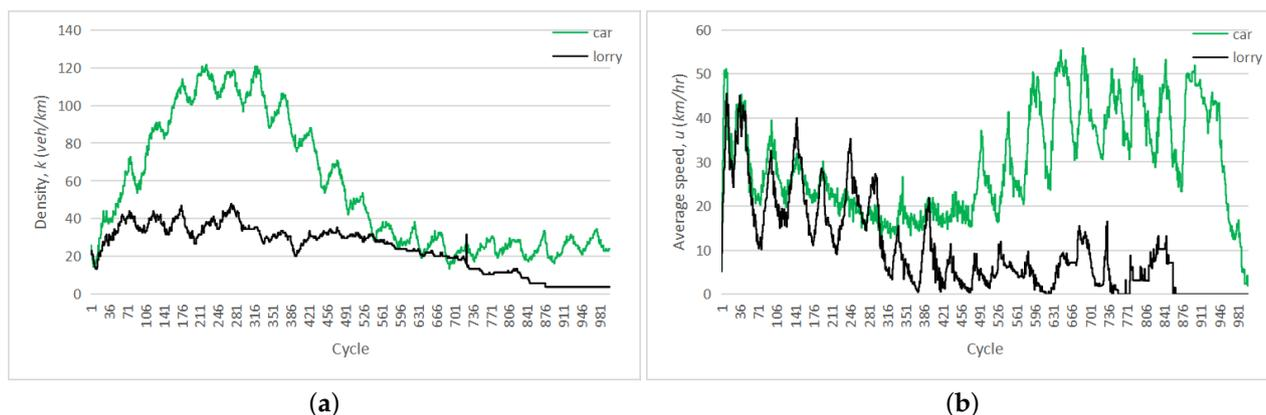
**Figure 8.** Time series density and average speed for two different types of vehicles on a homogeneous traffic flow. (a) Density of vehicles on the road for 1000 cycle. (b) Average speed of vehicles on the road for 1000 cycle.
