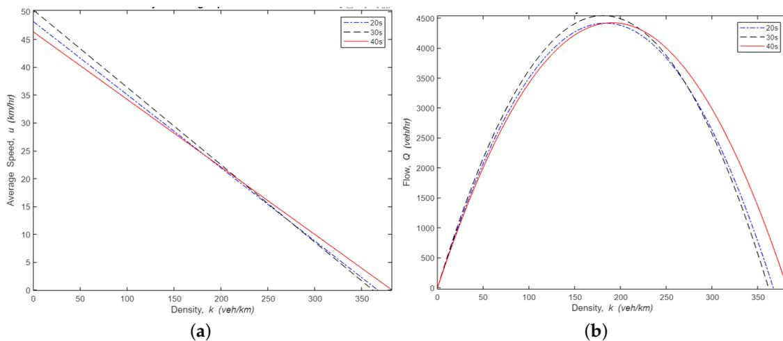
**Figure 19.** Speed-density and flow-density relation during the peak hour for different traffic light phasing. (a) Speed-density relation. (b) Flow-density relation.
