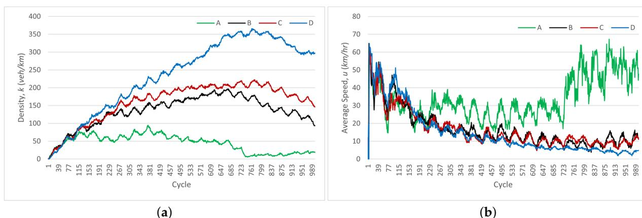
**Figure 11.** Comparison on the value of density and average speed for different vehicle composition. (a) Density against cycle. (b) Average speed against cycle.
