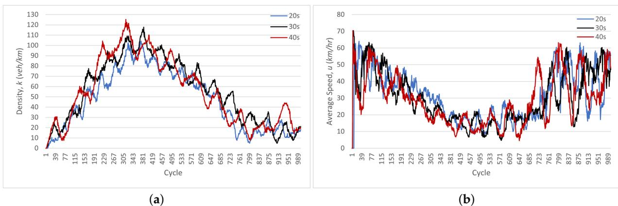
**Figure 20.** Comparison of the value of density and average speed over time during the peak hour for three different traffic phasing. (a) The value of density over time. (b) The value of average speed over time.
