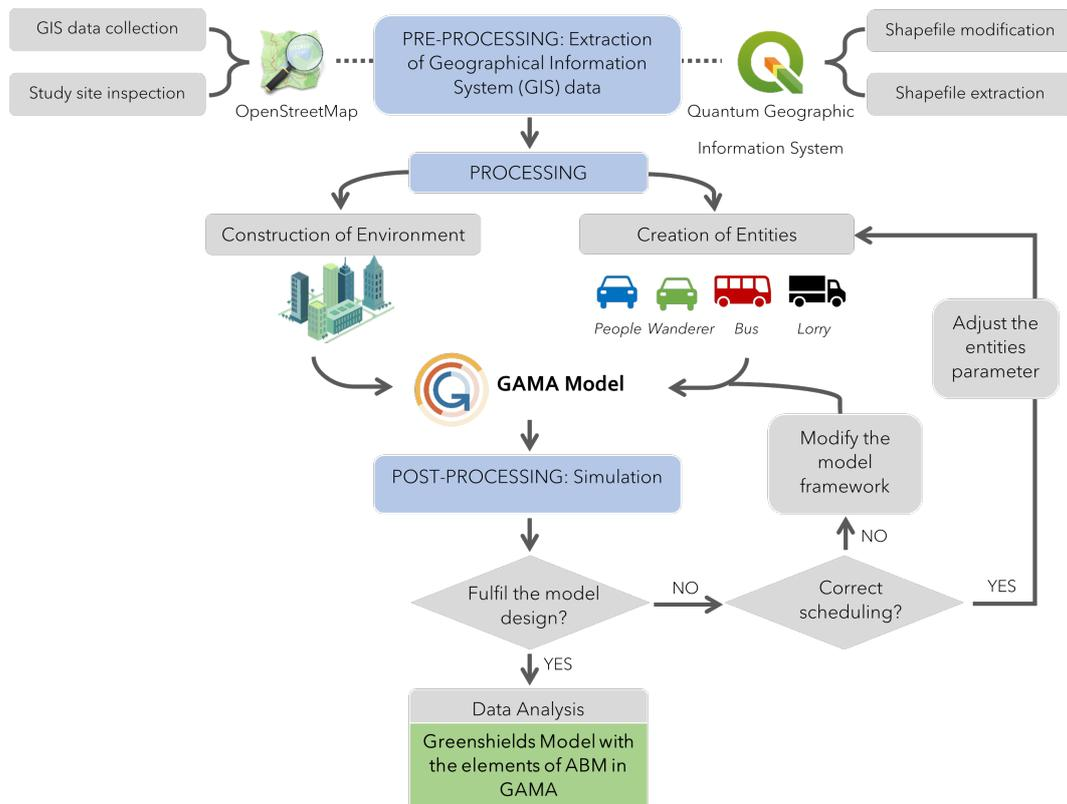
Figure 1. The flow of the proposed methodology.
