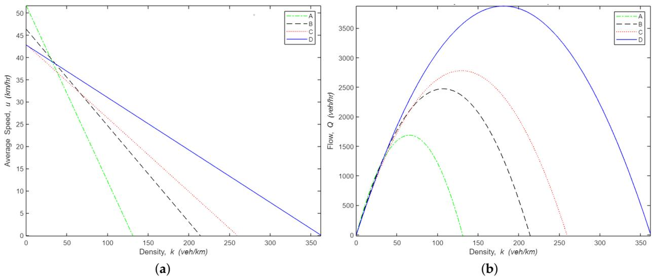
**Figure 12.** Speed-density and flow-density relation for different vehicle composition. (a) Speed-density relation. (b) Flow-density relation.
