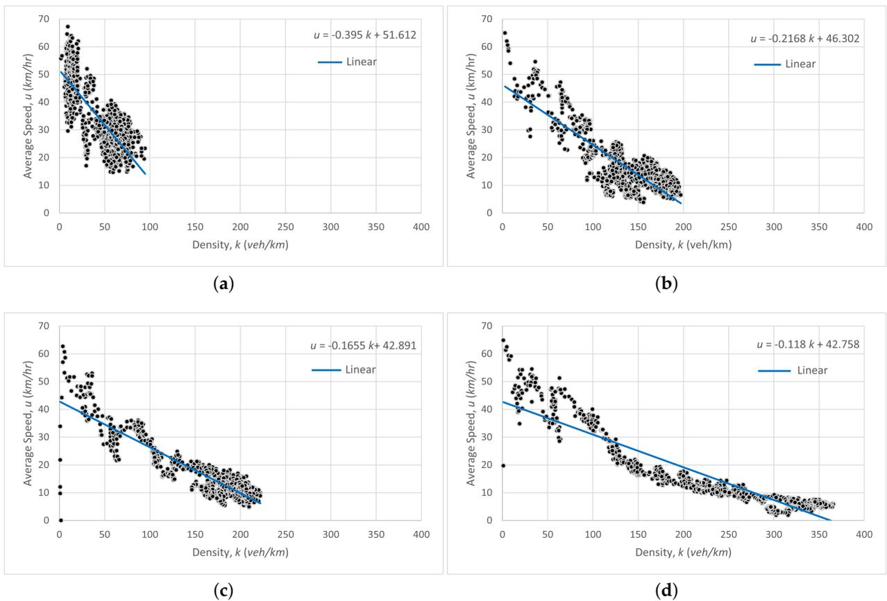
**Figure 10.** Results on the simulated data of density and average speed for simulation A, B, C and D. (a) Simulation A. (b) Simulation B. (c) Simulation C. (d) Simulation D.
