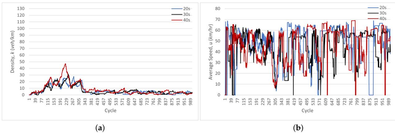
**Figure 16.** Comparison of the value of density and average speed over time during the off-peak hour for three different traffic phasing. (a) The value of density over time. (b) The value of average speed over time.
