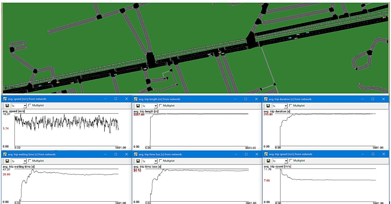
**Figure 9.** Simulation 3 and variations in different average travel time parameters and the average travel speed.
