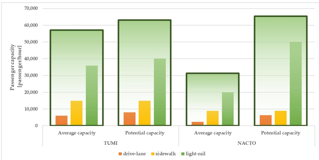
**Figure 6.** Expozitiei boulevard Section 2. Passenger capacity according to [71,72]. The green square represents the sum of the values from the orange, yellow and green bars. Elaborated by the authors.
