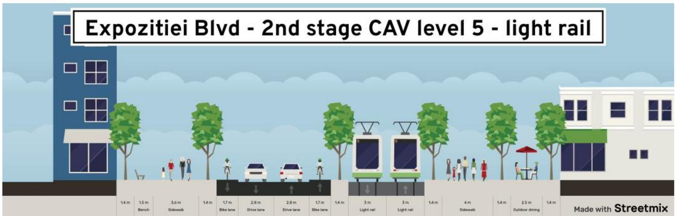
**Figure 16.** Expozitiei Blvd—Sectional view of the proposed changes in the second stage of Level 5 Avs—light rail/guided automated vehicle as a public transport service (designed using [67]).
