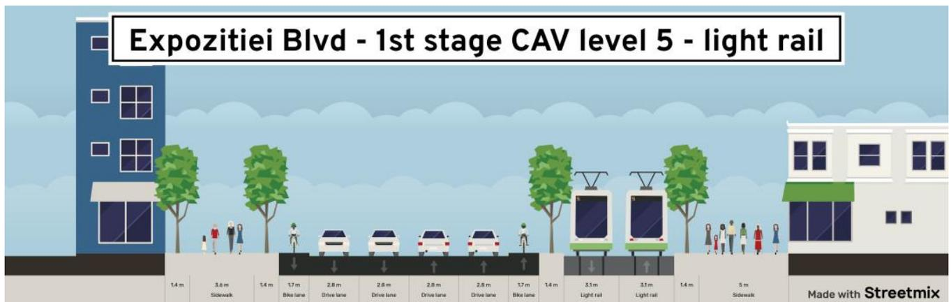
Figure 15. Expozitiei Blvd—Sectional view of the proposed changes in the first stage of Level 5 AVs—light rail/guided automated vehicle as a public transport service (designed using [67]).
