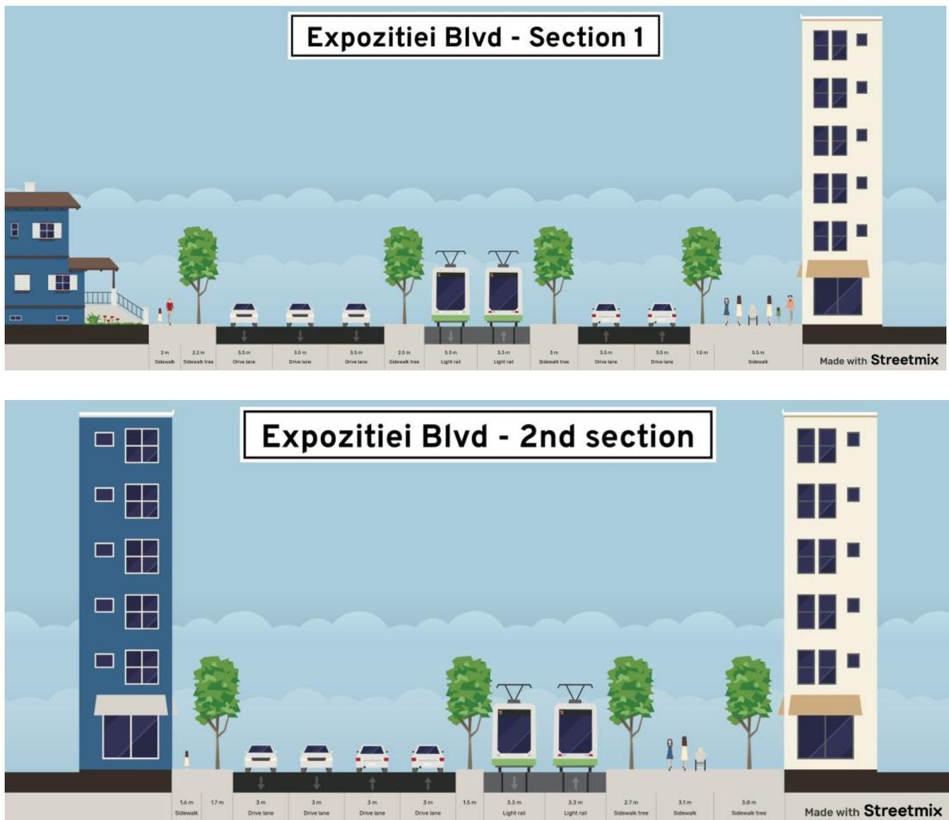
**Figure 4.** Geometric characteristics of Sections 1 and 2 developed using [67]. Elaborated by the authors.
