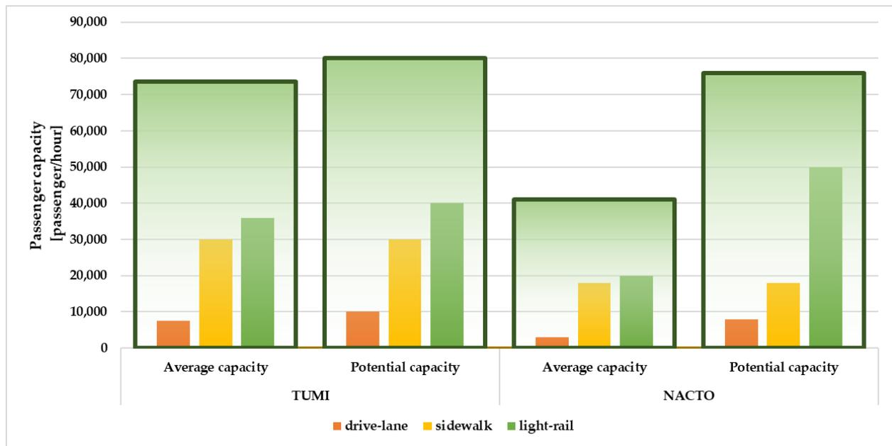
**Figure 5.** Expozitiei boulevard Section 1. Passenger capacity according to [71,72]. The green square represents the sum of the values from the orange, yellow and green bars. Elaborated by the authors.
