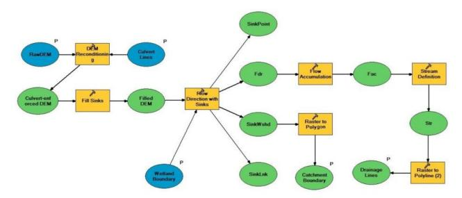
The above processes (Steps 1–7) were automated as a workflow in a ModelBuilder environment within an ArcGIS platform (Figure 2). ModelBuilder streamlined the processes and thus saved the execution time of running each function manually. Finally, the simulated catchment size, drainage channels and depression storage volumes resulting from the LiDAR-derived topography DEM and from the LiDAR-derived hydrologic DEM were compared based on our proposed method.
