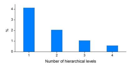
When more levels of abstraction are introduced, the number of processed nodes is further reduced. With a three-level hierarchy, the number of processed nodes is reduced to one-fourth of that of the 10-cell base level. As the path quality remains intact regardless of the number of hierarchical levels, the only drawback of using more hierarchies is the overhead incurred by the handling of several levels, which affects the preprocessing phase primarily.
