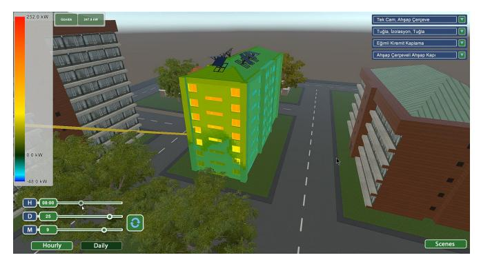
**Figure 3.** Estimation of the solar irradiation of buildings for a specific date and time. In this case the surrounding vegetation and the type of the receiving material is also taken into account in the estimations. (Image courtesy of Argedor).
