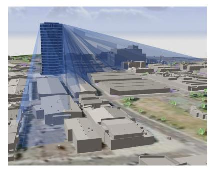
**Figure 5.** Estimating the shadow cast by a building for a few positions of the sun. For instance, this use case is valuable in assessing the effect that a proposed building design has on its surrounding. (Image courtesy of CyberCity 3D).
