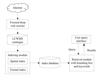
Figure 7. The LCWMS-SE architecture showing modules and linkages.
