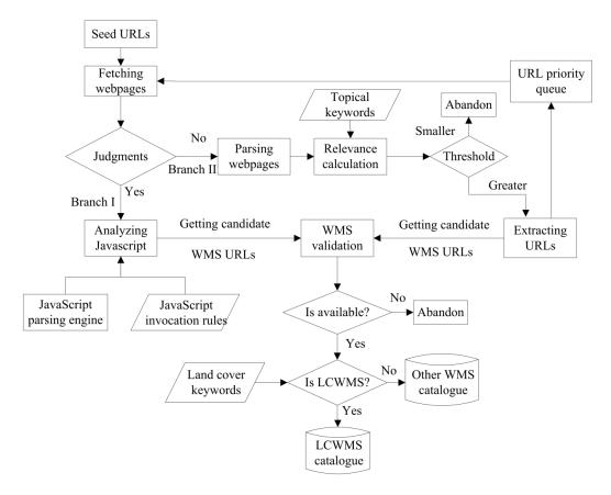
Figure 6. The framework of the focused deep web crawler for active discovery of LCWMSs.
