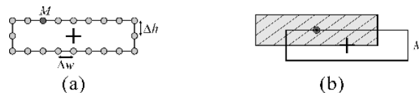
Figure 7. Schematic diagram of selecting the candidate label positions. (a) Reference points for distance computation; (b) generated candidate label position for reference point M .
