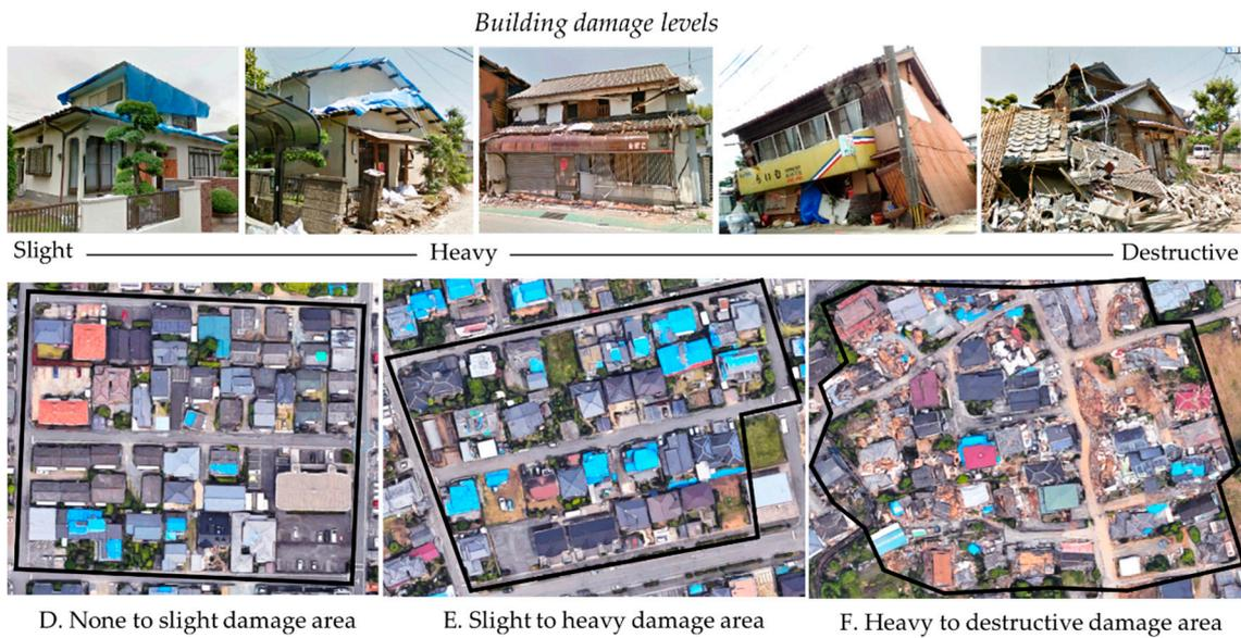
**Figure 6.** Examples of the urban damage degrees considered as ground truth for the accuracy assessment. Damaged areas were observed from Google Maps (2017). Field surveys and Google Street View after the earthquake also confirmed the damage levels. The locations of ground truth examples are provided in Figure 7.
