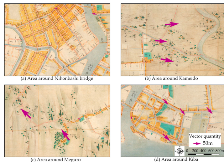
Figure 6. Directions of errors as compared with modern maps: (a) Area around Nihonbashi bridge; (b) Area around Kameido; (c) Area around Meguro; and (d) Area around Kiba (enlarged versions of Figure 5b with the equidistant cylindrical projection).
