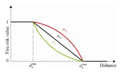
**Figure 5.** Defining a function to calculate the risk of high-risk urban infrastructures;  $d_{ij}^{max}$  shows the maximum effect distance,  $d_{ij}^{min}$  is the minimum impact distance; and  $\beta$  indicates how distance impacts the risk.
