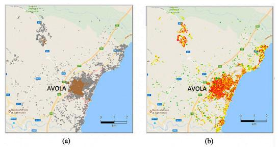
**Figure 4.** Territory of Avola. (a) Geographic Information System (GIS) data set: Masonry (brown) and reinforced concrete (grey) buildings; (b) initial vulnerability map: Low (green), medium (yellow) and high (red) vulnerability buildings.
