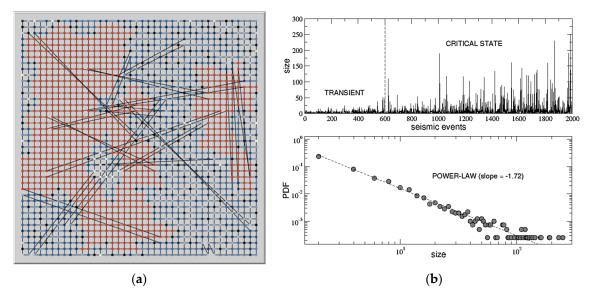
**Figure 2.** (a) The small world lattice of the OFC model; (b) The sequence of earthquakes' sizes in the transient and in the critical state (upper panel) with the corresponding probability distribution (lower panel).
