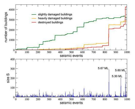
**Figure 7.** Bottom panel: A simulated sequence of 1000 seismic events (100 per day). Top panel: Evolution of the corresponding number of slightly damaged, heavily damaged and destroyed buildings for  $f_B = 0.4$ .
