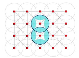
**Figure 6.** Overlapping circles around the active nodes. Inside these circles, only a fraction  $f_{\rm B}$  (control parameter) of buildings will be considered for the damage evaluation.
