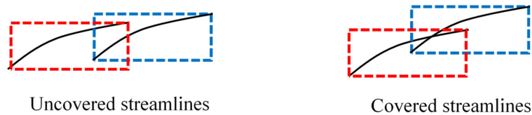
Figure 3. Schematic diagram of two kinds of streamline encased rectangular covering situation. The left image represents a case where the streamlines do not conflict, and it should not be excluded. The right-hand image is one that represents conflict, and it should be excluded.
