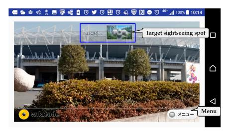
Figure 8. Interface of object-recognition AR screen.
