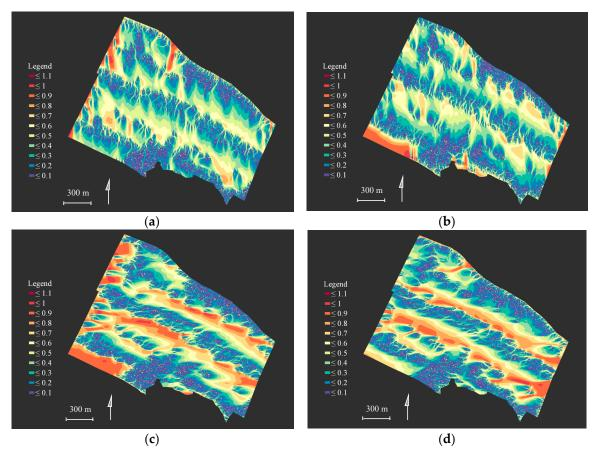
**Figure 7.** Visualization of relative wind speed: (**a**) north wind, (**b**) south wind, (**c**) west wind, and (**d**) east wind.
