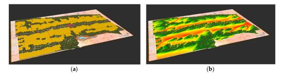
**Figure 6.** Computational fluid dynamics (CFD) analysis of 3D models: (**a**) reconstruction of Kichijoji village and (**b**) CFD analysis results over the reconstruction.
