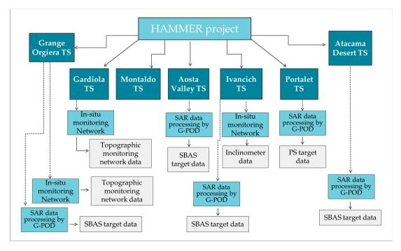
**Figure 7.** H-SDI metadata hierarchy scheme based on "Parent/Child" links; in dark blue are the test sites of the Hammer project; in blue are the available sensors and/or in situ instruments for each test site; in light grey are the raw data of ground deformation measurements.
