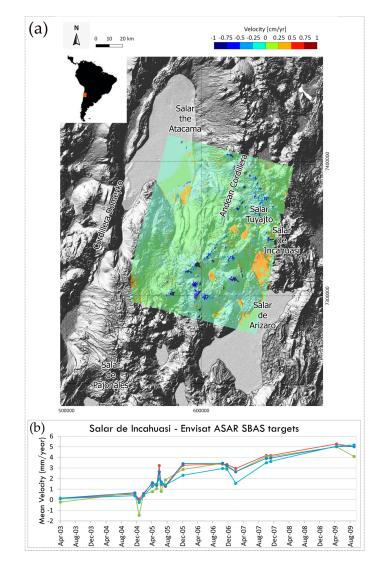
**Figure 12.** Example of data usage: (**a**) map of the SBAS targets, processed by G-POD, generated in GIS environment for the Salar de Atacama test site; (**b**) plot of the ground deformation time-series relative to some SBAS target of the Salar de Incauasi, located in the Salar de Atacama AOI.
