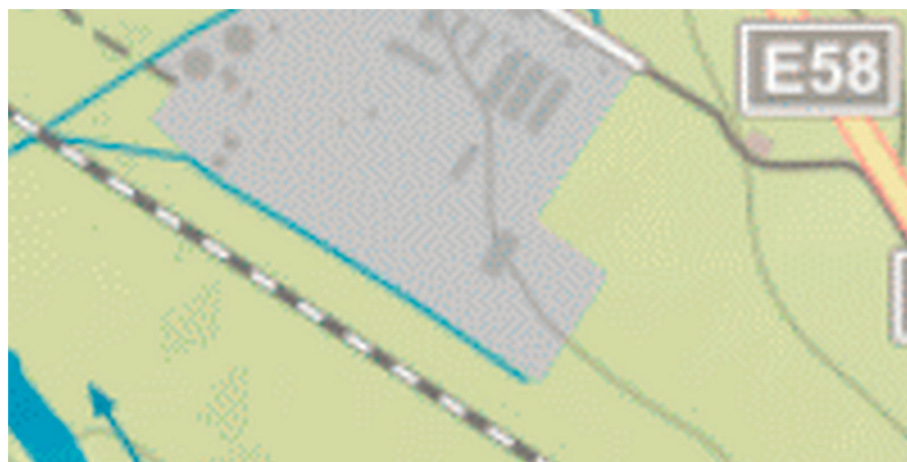
Figure 15. Dotted structures caused by colour depth reduction in the case of M4.
