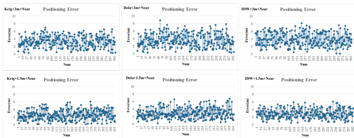
Figure 12. Positioning error with the different interpolation methods (IDW and Delaunay) and interpolation densities (3 and 1.5 m) considering the near relation.
