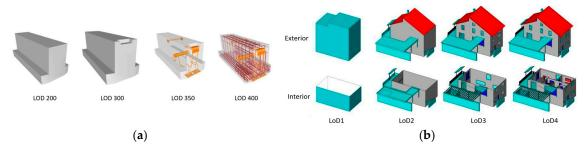
**Figure 2.** Different LODs in IFC for a precast structural inverted T beam (extracted from <a href="https://bimforum.org/lod/">https://bimforum.org/lod/</a>) (a) and LoDs for CityGML of a residential building (courtesy of Karlsruhe Institute of Technology) (b).
