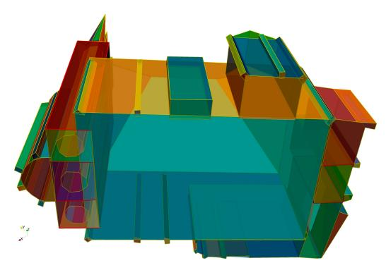
Figure 4. Example of non-consistent CityGML data.
