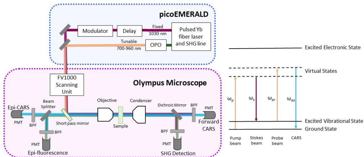
**Figure S1.** Simplified schematic of microscope set up and corresponding energy diagram of CARS process.
