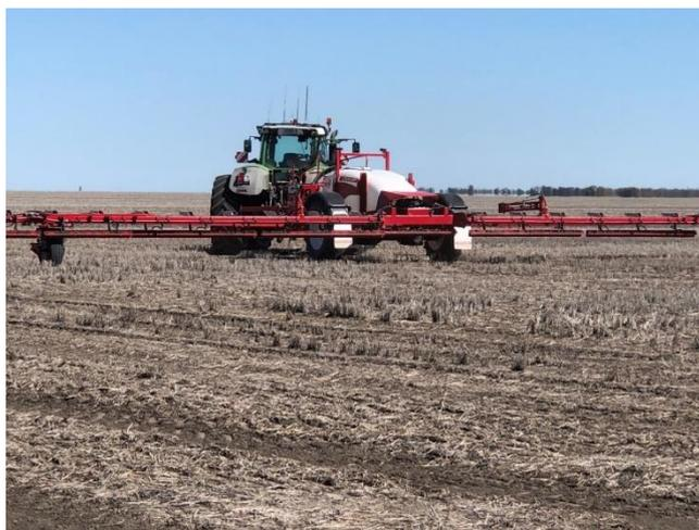
**Figure 3.** Autonomous site-specific weed control with a real-time weed detection and application sprayer in a fallow field.
