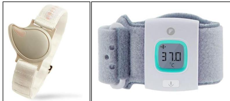
**Figure 1.** Wearable body temperature assessment devices.
