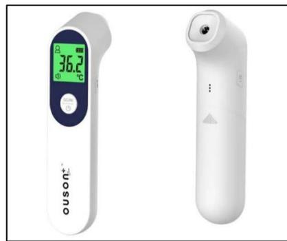
Figure 10. Non-contact thermometer.
