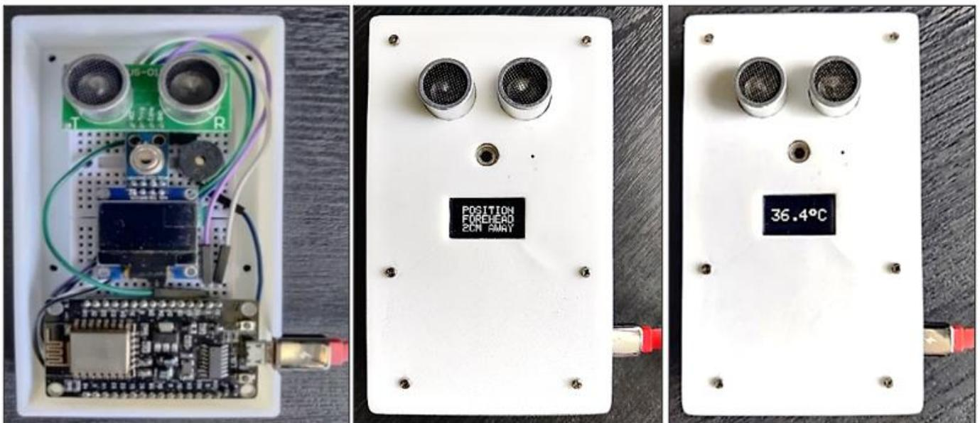
**Figure 6.** Assembly of the body temperature screening system.
