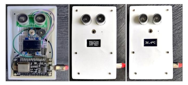
Figure 6. Assembly of the body temperature screening system.
