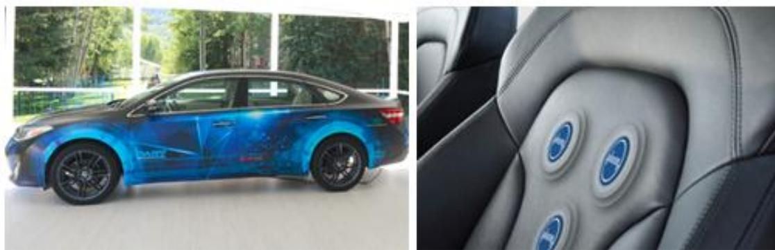
**Figure 4.** Toyota’s DARV 1.5 and Plessey’s EPIC Seat Sensors. Image credit: Toyota’s Collaborative Safety Research Center [42] and the Motor Report [43].
