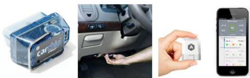
**Figure 9.** DIYdiagnostics: CarChip Connect and Automatic Link. Image credit: Davis Instruments [77] and Automatic [78].
