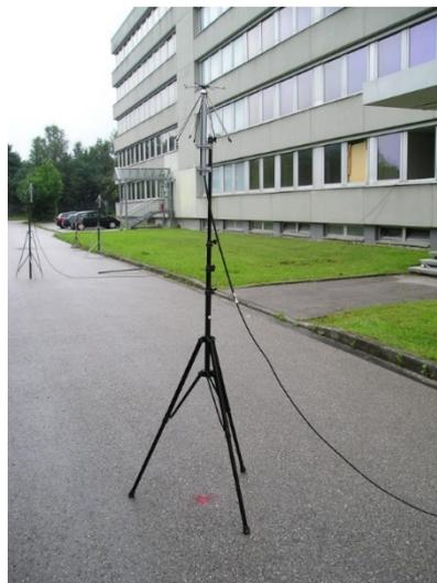
**Figure 20.** Transmitters during setup and deployment outside the test building.
