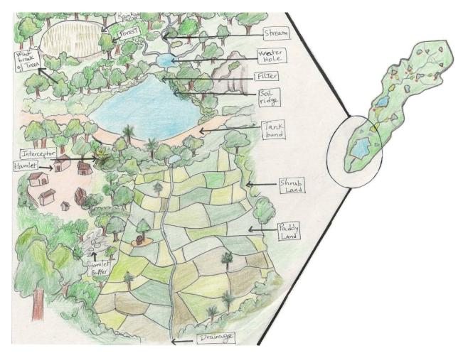
Figure 1. Main components of the tank.
