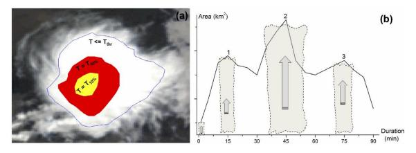
**Figure 1.** (a) A convective cloud cell as delimited through Meteosat imagery (Kolios, 2009). The red and yellow colored internal areas depict very cold isotherms where active convection can occur; (b) Schematic representation of the fluctuations regarding the cloud top areal extent during a typical MCS lifecycle. of the areal extent. Any of the local maxima that fulfill the criterion of the equation 1 was considered capable of producing CGWs.
