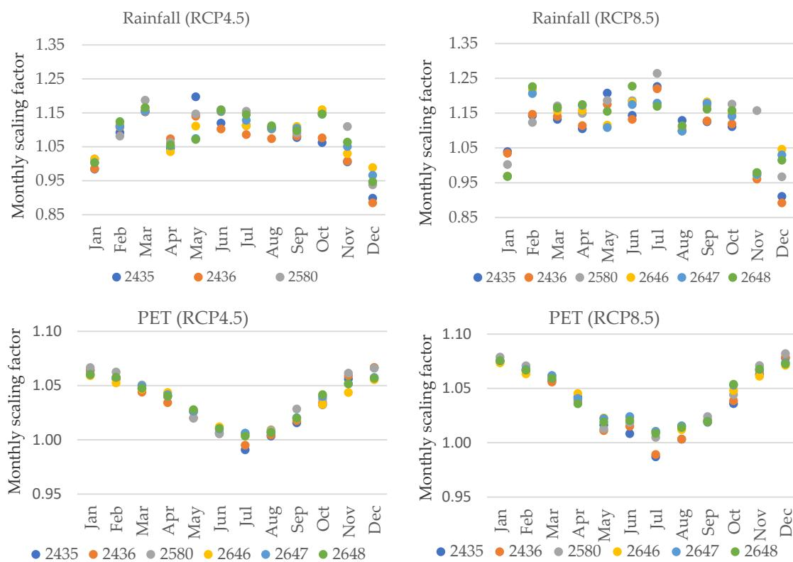
**Figure 9.** Variations of monthly scaling factor of rainfall (**upper panels**) and PET (**lower panels**) across the northwest region for the six GCM grids (refer to Figure 3 for location).
