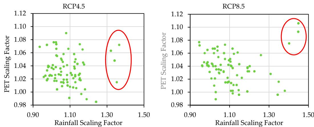
**Figure 6.** Scatter plot of modelled scaling factors for rainfall and PET for 28 GCMs for the six GCM grids. Red circles show the outliers in model projections.
