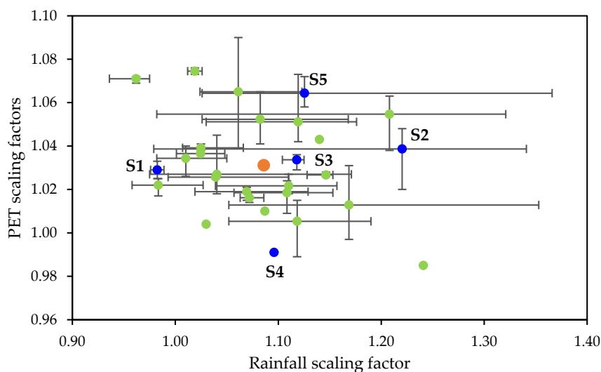
**Figure 5.** Method of selecting best GCMs for five scenarios (S1 to S5). Green, blue and orange dots represent 28 GCMs, five selected GCMs for S1 to S5 and average of 28 GCMs respectively. The error bar shows the spatial variability between six grids.
