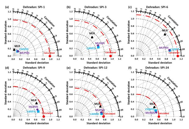
Figure 12. (a-f) Taylor diagram of predicted and calculated multi-scalar SPI at Dehradun station.
