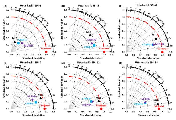
Figure 17. (a-f) Taylor diagram of predicted and calculated multi-scalar SPI at Uttarkashi station.
