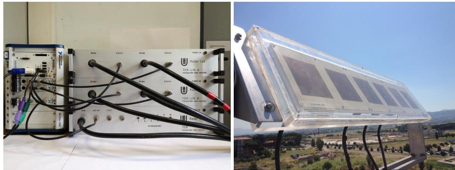
**Figure 4.** Transponder Data Recorder (TDR) system pictures: on the left the TDR receiver, on the right the TDR antenna.
