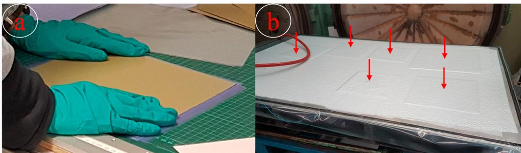
**Figure 11.** (a) Hand lay-up of the GLARE stack; (b) breather fabric and air-tight plastic foil covering the GLARE panels on the stainless-steel bed of the autoclave prior to curing; red arrows indicate the location of GLARE panels on the autoclave bed.
