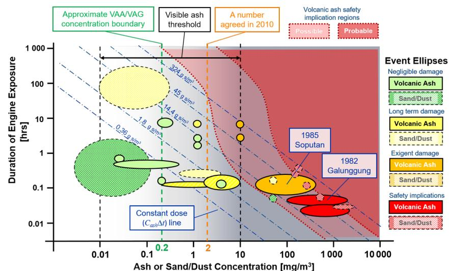
**Figure 2.** The Duration of Exposure versus Ash Concentration (DEvAC) chart, showing the two encounter events being investigated and their corresponding concentration and duration ranges [5].
