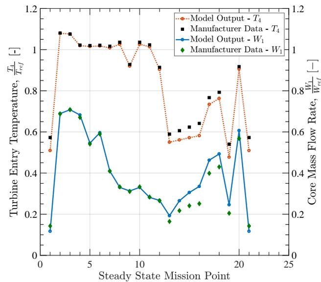
**Figure 3.** Validation of the RB211-524C NPSS engine performance model for turbine entry temperature and core mass flow rate.
