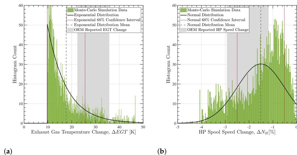
**Figure 6.** Model predicted change in exhaust gas temperature (a) and high-pressure spool speed (b) for the Mount Galunggung encounter event, with exponential and normal distributions, respectively, fit to the data and a comparison between the mean performance change predicted by the model and the range observed for the four engines involved in the event.
