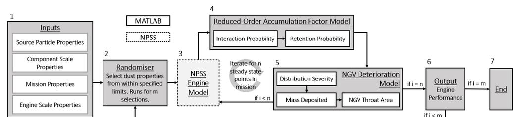
**Figure 4.** Block diagram showing the structure of the coupled degradation model used to carry out the statistical analysis of dust properties for dust cloud encounter events. Step numbers in the model process are indicated above each block.
