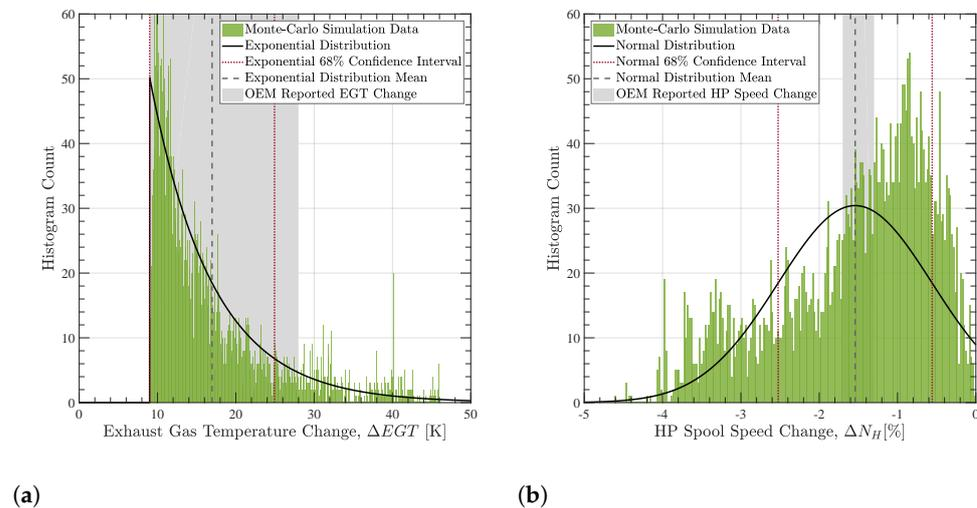
**Figure 7.** Model-predicted change in exhaust gas temperature (a) and high-pressure spool speed (b) for the Mount Soputan encounter event, with exponential and normal distributions respectively fit to the data and a comparison between the mean performance change predicted by the model and the range observed for the four engines involved in the event.
