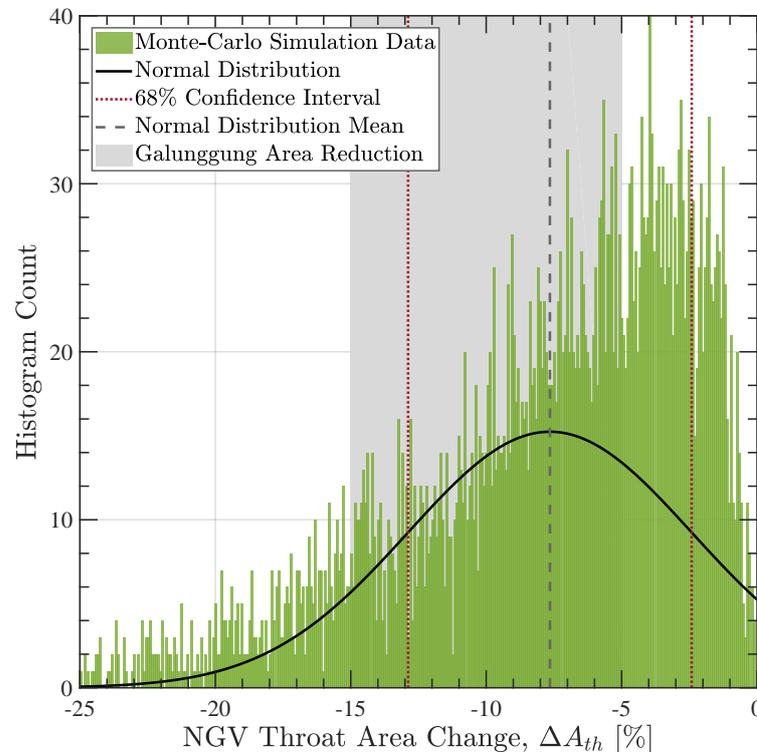
**Figure 8.** The predicted NGV throat area reduction for the Soputan encounter during which engines did not surge, indicating how this was comparable to that observed for the Galunggung event in which all four engines experienced surge.
