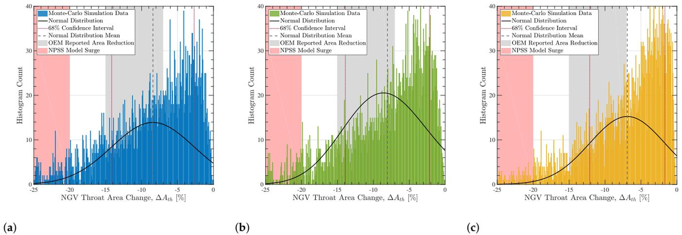
**Figure 5.** Predicted high-pressure turbine throat area change distributions for particle sphericities of (a)  $\phi = 1.00$ , (b)  $\phi = 0.75$  and (c)  $\phi = 0.54$  comparing the predicted mean throat area change and 68% confidence interval with observations from the four engines involved in the Galunggung event.
