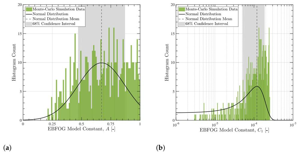
**Figure 9.** Histogram of outputs showing the distribution of input values for the empirical constants  $A$  (a) and  $C_1$  (b) that resulted in a simulation predicting both EGT rise and HP speed reduction that fall within the ranges observed during the Galunggung encounter event. The predicted mean value from the simulations carried out and the confidence interval for this prediction are also presented.
