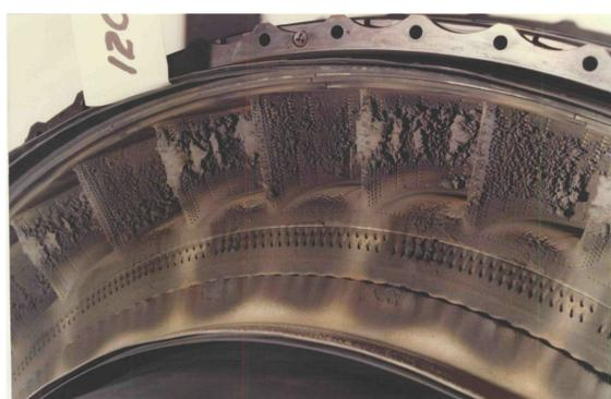
**Figure 1.** Deposited volcanic ash on the high pressure turbine nozzle guide vanes of a Rolls-Royce RB211-524C engine involved in an encounter with the volcanic ash plume from the 1982 eruption of Mount Galunggung in Indonesia [14].
